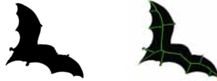
Figure 2: Left: a view of a bat. Right: the shock graph constructed from the medial axis and superimposed on the left image.
