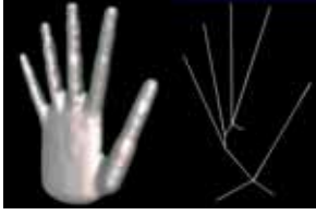
Figure 3: The Reeb graph constructed for the object on the left is shown on the right.
