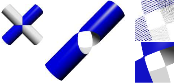
Figure 7: A difficult boolean difference operation.
