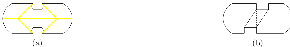
Figure 4: Problems with the short-cut rule; (a) selecting closest boundary points, (b) selecting closest cusps
