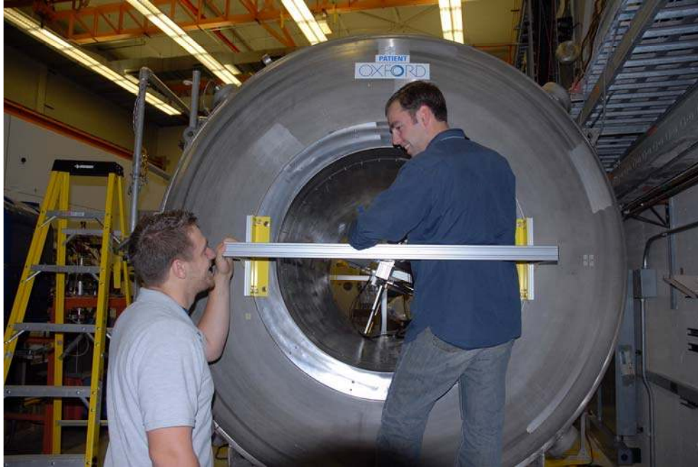
Figure 1 Western Michigan University graduate student Jonathon Lighthall (right) and undergraduate student Jack Winkelbauer (left) adjust a field mapping apparatus in the HELIOS spectrometer magnet at the ATLAS accelerator facility at Argonne National Laboratory.
