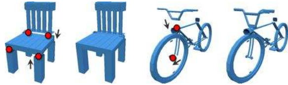
Figure 13: The synthesized models can be further refined using docker-based part deformation. In these examples, the parts of the chair and bike are brought back into contact based on nearest part dockers.
