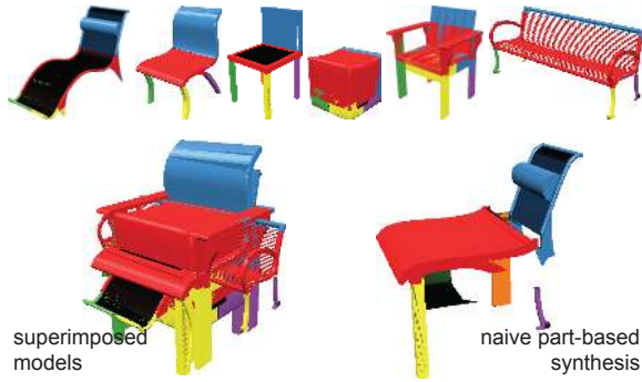
Figure 4: Combining a random selection of chair models (top), even when they are consistently segmented, is challenging. The models have different proportions of parts, that make a part selection based on visual inspection of the superimposed models (bottom-left) confusing and can easily result in meaningless part ensembles (bottom-right). Instead, we expose a constrained and intuitive part-based shape space for easy exploration and synthesis.
