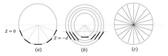
**Figure 7.** Different coil arrays configurations proposed in [75]: (**a**) hemispherical; (**b**) plane and (**c**) torus array.
