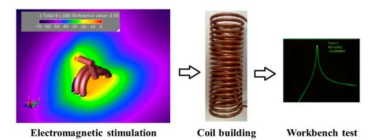
**Figure 4.** Different steps of inductors development for hyperthermia applications. Numerical design is followed by fabrication and workbenching tests.
