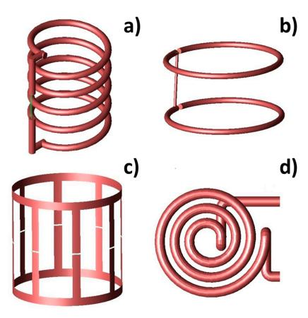
**Figure 3.** Sketch of the typical coil configurations employed in hyperthermia experiments: a solenoid (**a**), Helmholtz configuration (**b**), birdcage (**c**) and pancake (**d**) coils.
