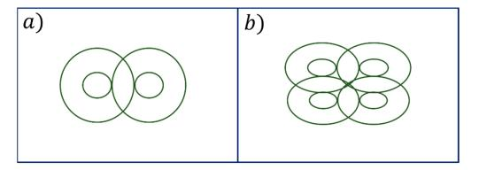
**Figure 6.** Perspective view of TMS figure-of-eight enhanced coils configurations (**a**), and the "four leaf solution" (**b**) [72].
