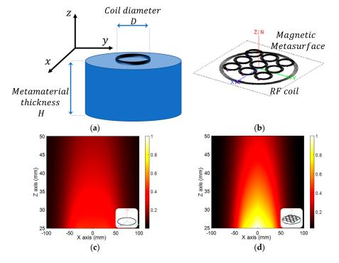
filtering or focusing elements. In this sense, an array of split rings or spiral resonators are the most suited unit-cells to interact with the RF magnetic field (Figure 9a,b).
