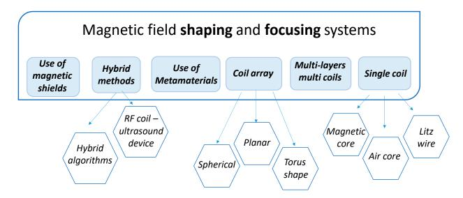
Figure 1. Scheme of the radiating solutions for magnetic field shaping classified by the adopted approach.
