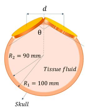
Figure 5. Biconical stimulator coils system: pictorial representation.
