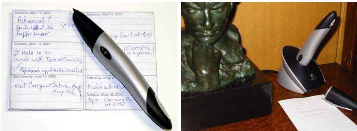
Fig 12: The grandparents write on their small pocket calendar printed on digital paper (left) and replace the pen on the cradle to transfer the information to the computer (right).
