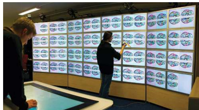
Figure 1. The WILD room: 32-monitor wall display showing 64 brain scans, multi-touch table, motion tracking system.
