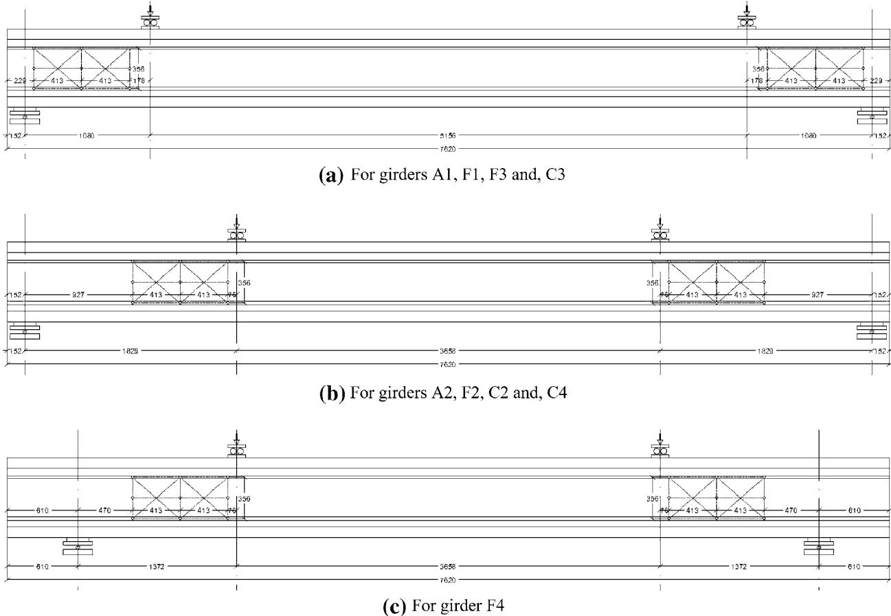
**Fig. 3** Locations of applied actuator loads and support reactions. **a** For girders A1, F1, F3 and, C3. **b** For girders A2, F2, C2 and, C4. **c** For girder F4 (All dimensions are in mm).
