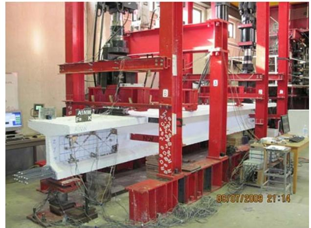
**Fig. 4** Test set up for girders.
