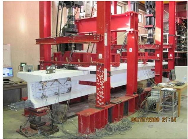
Fig. 4 Test set up for girders.
