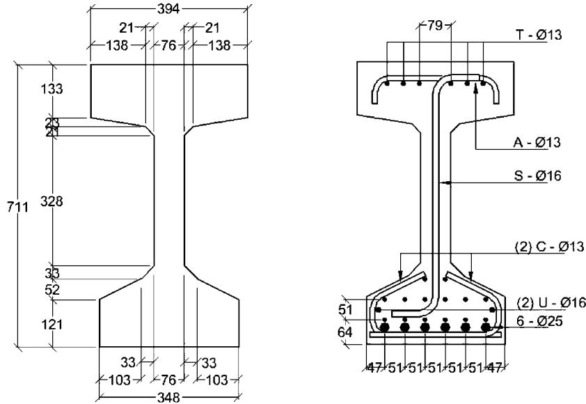
**Fig. 2** Cross-section and reinforcement details for modified Tx28 Girders C2 and C4 (All dimensions are in mm).
