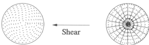
Figure 1. Schematic of special sample preparation and shear experiment. The planar extension orients the PS cylinders in the extension direction within a rectangular sheet from which a circular sample is pieced together and sheared. The dashed lines represent the local direction of PS domains. Real samples show a fluctuation of the director (see X-ray pattern, Figure 3).
