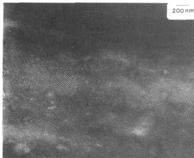
Figure 10. Electron micrograph from a cut perpendicular to the 3 axis, the sample radius at \gamma = 2.8 . There is a majority of cylinders lying end-on, indicating they are still parallel to the sample radius (initial order), and some are already lying more edge-on, indicating they are at an angle to the sample radius.
