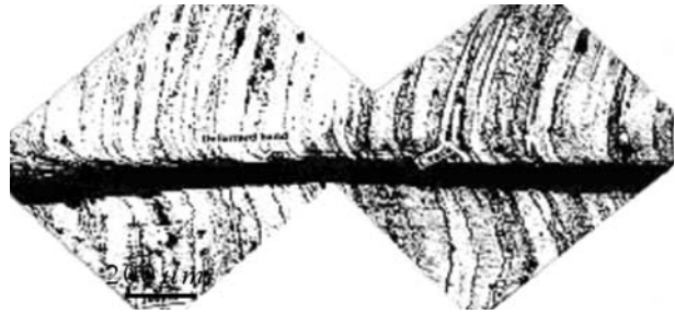
Fig. 34—Fracturing along the shear bands in Al-Li alloy subjected to dynamic impact compression.
