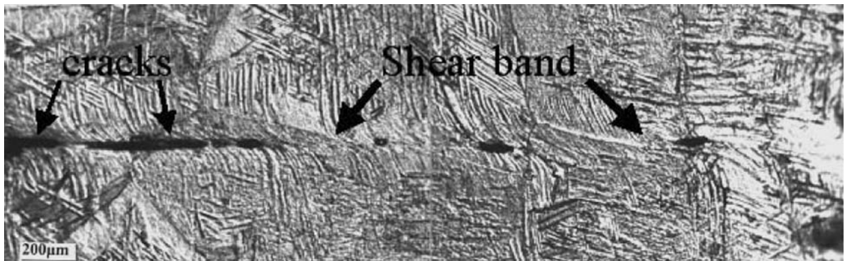
Fig. 5—Shear band transverse several grains and coalescence of microcracks along the shear band during localization in Ti-6Al-4V alloy.
