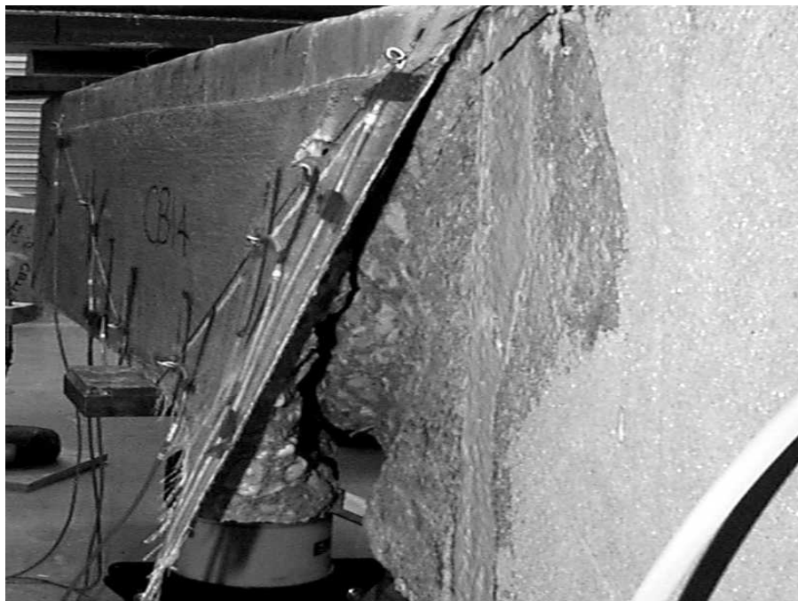
Figure 6: Failure Pattern of the Beam Bonded with CFRP Fabric Inclined at 90° and 0°; Rupture and Delamination of CFRP Fabric
