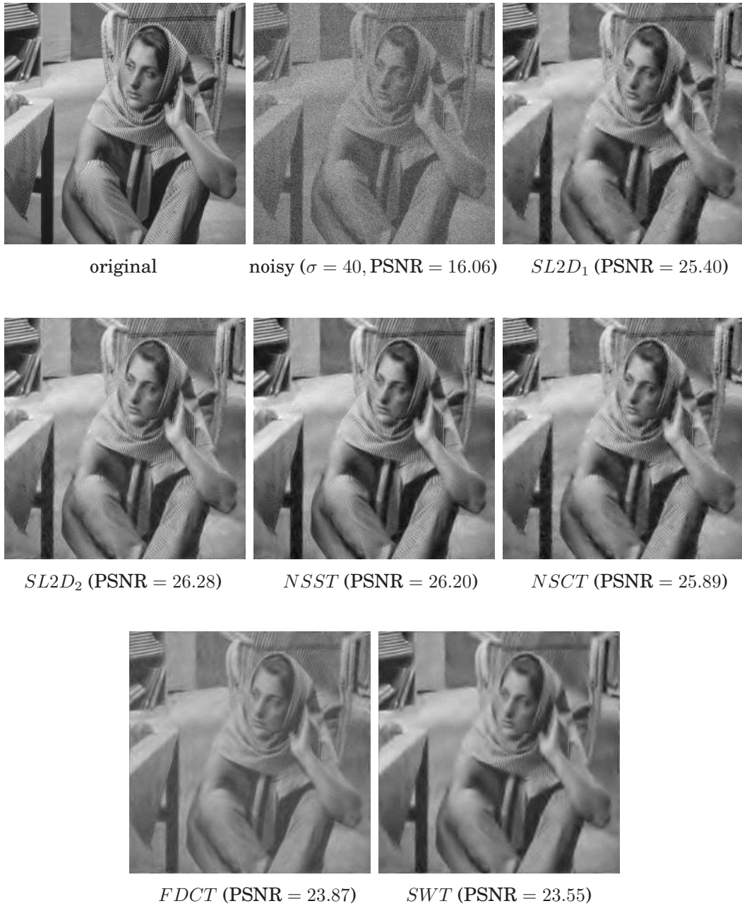
Fig. 19. The Barbara image is distorted with Gaussian white noise with \sigma = 40 and denoised using various sparse approximation schemes.
