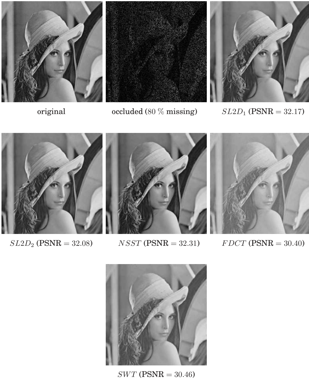
Fig. 20. The Lenna image is occluded with a random binary mask and denoised using various sparse approximation schemes.
