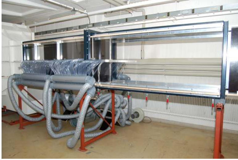
FIGURE 4.1. Photograph of the test-section situated in the Boundary Layer (BL) wind tunnel.
