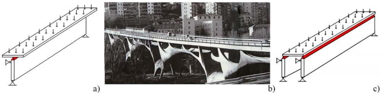
Figure 9: Unstable straight deck (a); Stable straight deck (b) and (c)
