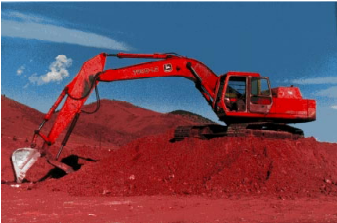
Figure 16. A small hydraulic shovel with a special gripping attachment on the bucket. Note the ability to dig below grade.
