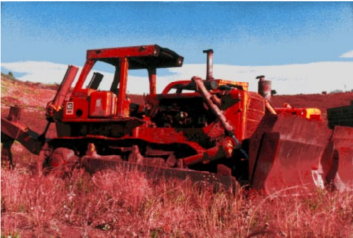
Figure 10. This model of dozer has an operating mass of nearly 37,000 kg, a height of 3.4 m, a length of 6.2 m, and a width of 3.4 m (excluding blade). Blade capacity varies from 4.7 m 3 to 11.7 m 3 , depending on blade configuration (data from Caterpillar [7]).
