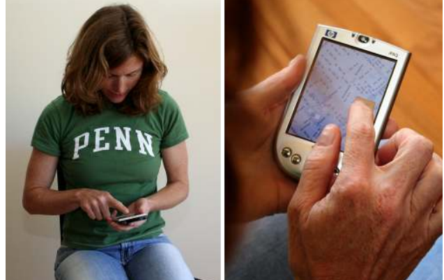
Figure 10. Apparatus: participants acquired targets on an IPAQ 4100 PDA using their index finger.
