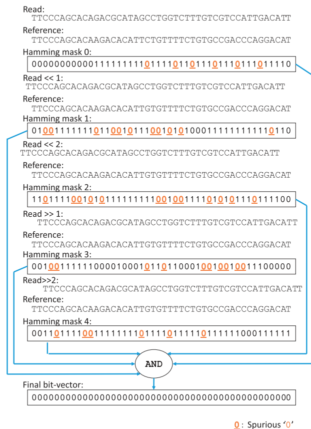
Fig. 2. An example of an incorrect mapping that passes SHM. In this example, during the bit-wise AND operations, short streaks of ‘0’s at different locations in the Hamming masks overwrite (mask out) any ‘1’s in other Hamming mask that are at the same locations. As a result, the final bit-vector of SHM is full of ‘0’s. With SRS, streaks of ‘0’s that are shorter than three are marked as spurious and are subjected to removal later on
