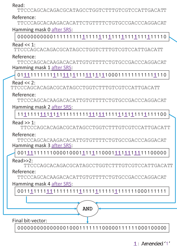
Fig. 3. The incorrect mapping from Figure 2 is filtered correctly by SRS, since most of its short streaks of ‘0’s are turned into amended ‘1’s. Amended ‘1’s transparent during the AND operations
