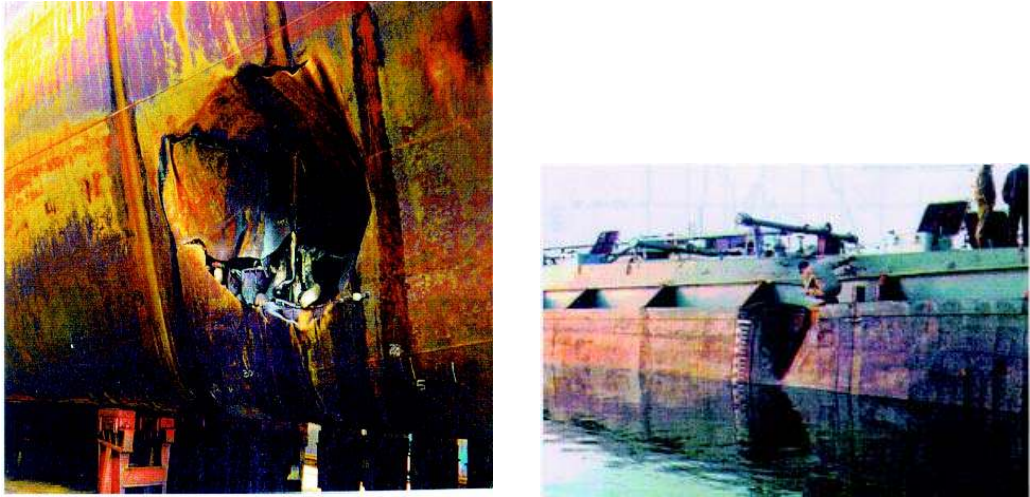
Figure 4.2: Imprints on side of struck vessel, left bulb, right bow.
