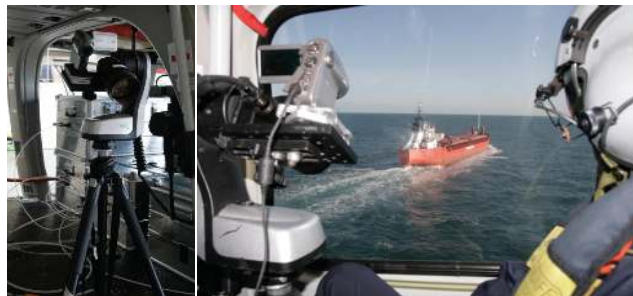
Fig. 8. Measurement setup in a Dauphin helicopter used in the North Sea campaign. The picture shows the telescope with a video camera for documentation on the side. The aluminium box in the bottom right of the picture contains the spectrometer. The other boxes contain in situ gas analysers. The same system was used in the CASA-212 airplane in the Baltic Sea.
