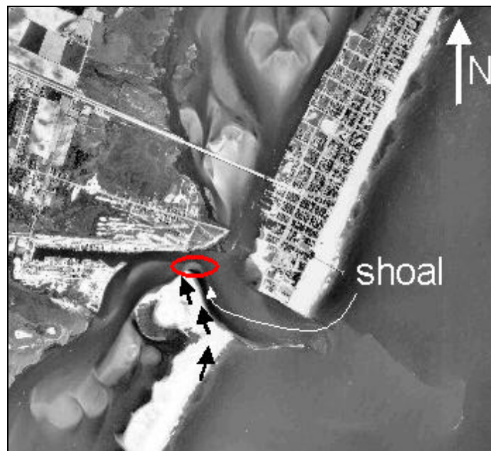
Figure 4a. Ocean City Inlet, Maryland with sediment-transport pathways over and through jetty (based on Dean and Perlin (1977); photograph dated 8 June 1952)
