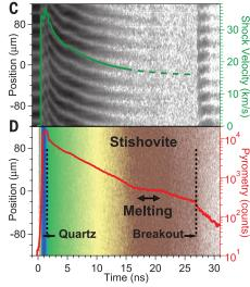
associated with the threshold in electrical conductivity. Melting is evident from a thermal anomaly attributed to latent heat and seen here as a change in the decay of the Hugoniot temperature and the recovery of VISAR fringes upon breakout into vacuum (5).
