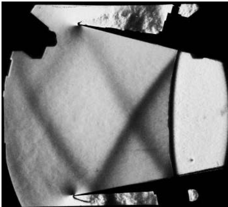
FIGURE 27. Outgoing shock in \text{CO}_2 . Reflected shocks in the lower Mach number case are fully dispersed.
