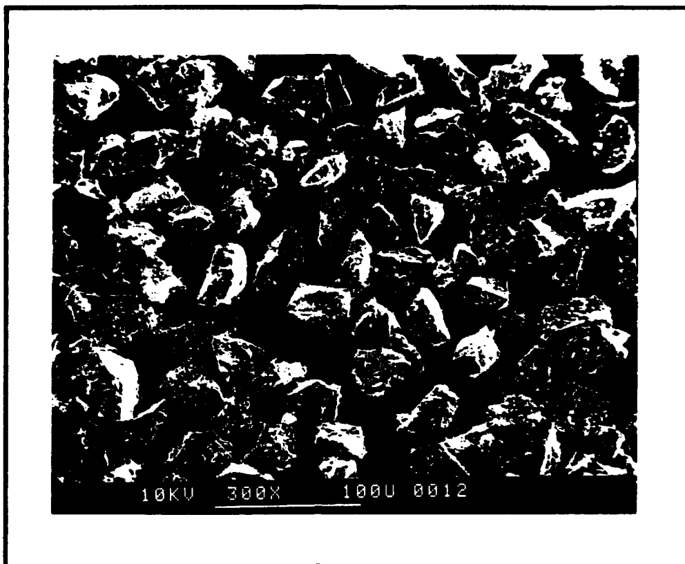
Figure 3.10 Scanning Electron Microscope photomicrograph of crystalline boron sieved between 20-25 microns. The long bar at the bottom of the photograph is 100 \mu\text{m} .
