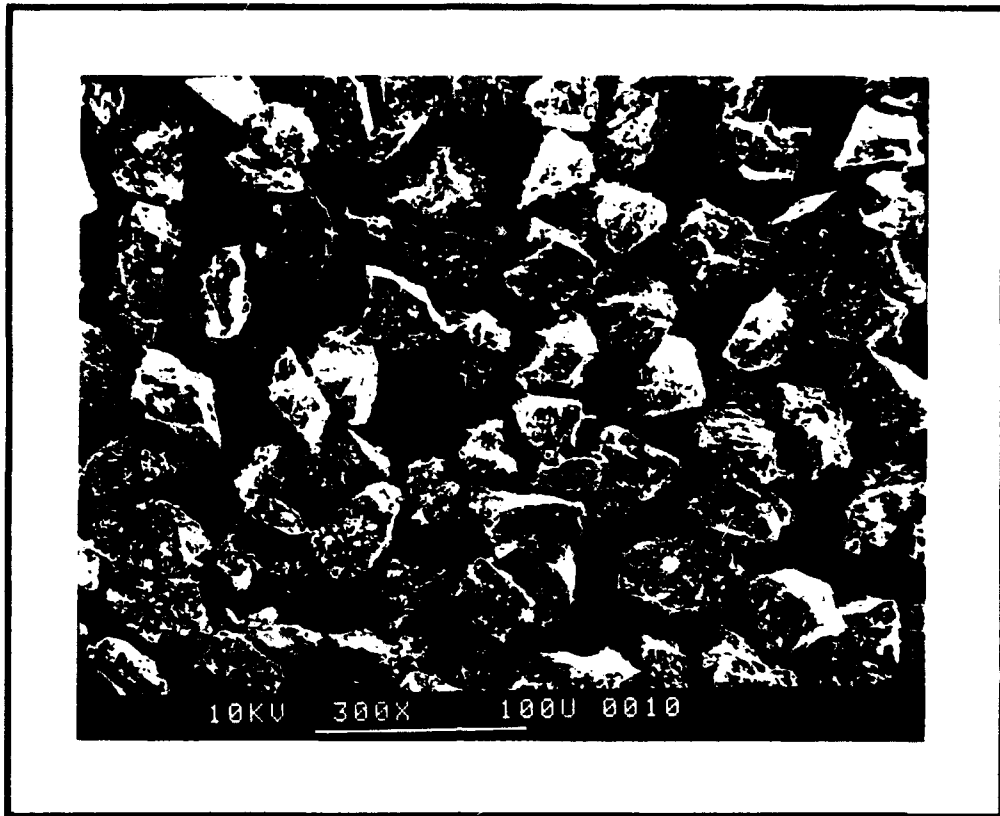
Figure 3.12 Scanning Electron Microscope photomicrograph of crystalline boron sieved between 25-32 microns. The long bar at the bottom of the photograph is 100 \mu\text{m} .
