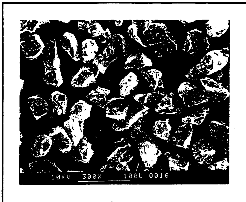
Figure 3.14 Scanning Electron Microscope photomicrograph of crystalline boron sieved between 32-38 microns. The long bar at the bottom of the photograph is 100 \mu\text{m} .
