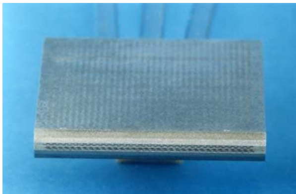
Figure 5. Front view of cowl leading edge model showing gas jet nozzles.
