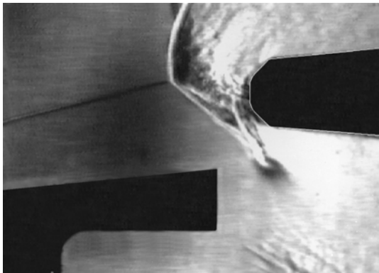
(a.) Modified Type III shock interference before transition ( Y=0.438 in.)
