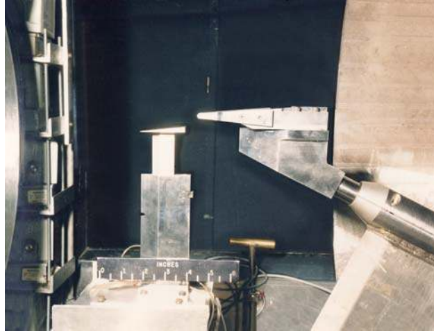
Figure 7. Model and shock generator installed in the test section of the NASA Langley 15-Inch Mach 6 High Temperature Tunnel.
