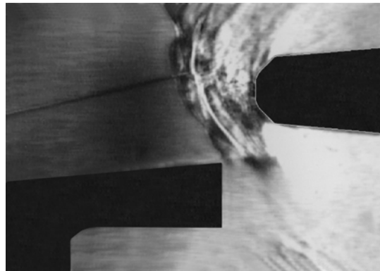
(b.) Modified Type IV shock interference after transition ( Y=0.430 in.)
