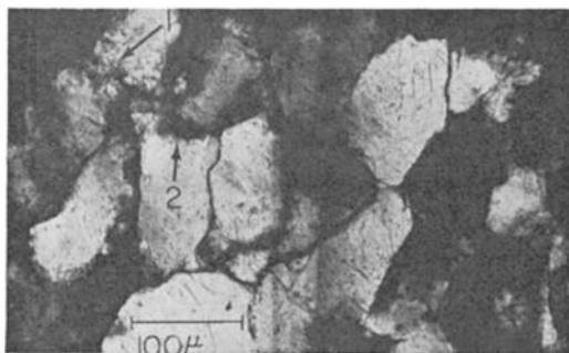
Fig. 7. Photomicrograph (crossed Nicols) showing jigsaw texture due to plastic deformation of quartz grains on a class 2 rock. Center grains have re-entrants on boundaries due to deformation. Arrows point to symplektic region (1) and to isotropic region (2) on grain boundary. The isotropic region probably contains an unresolvable mixture of coesite and diaplectic glass. Cleavages are visible on the grains. Emulsion is streaked in center of photograph.
