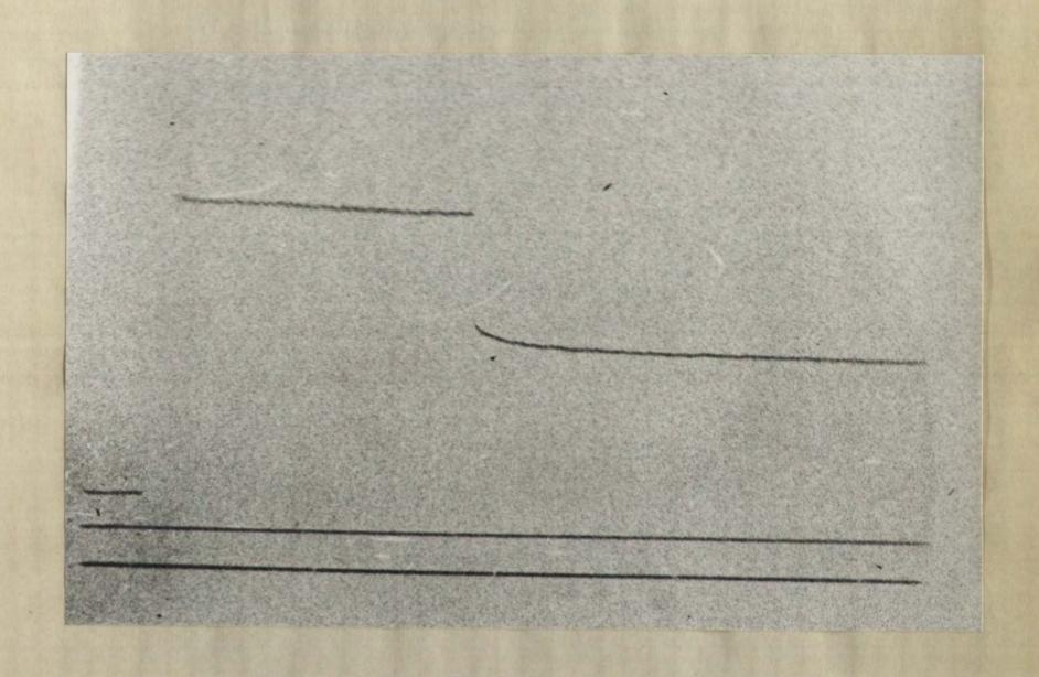
Fig. 4. A typical oscilloscope record of the change in x ray transmission across a shock in a 95% Xe - 5% O mixture at an initial pressure of 1.99 cm Hg. The three sweep traces from top to bottom are the x ray signal, a base line, and 100 µsec timing marks. Shock velocity was 1.229 mm/µsec.
