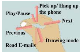
Figure 3: 3D radial gesture set (Left, Right, Front, Back, Up, Down) mapped to frequent actions on a smart phone.
