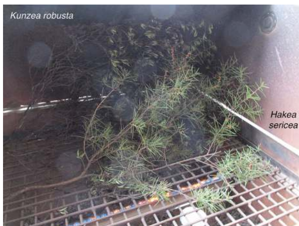
Figure 1. Samples of Hakea sericea and Kunzea robusta arranged on the grill. The gas burner beneath the grill is preheating the samples prior to ignition of the blowtorch.
