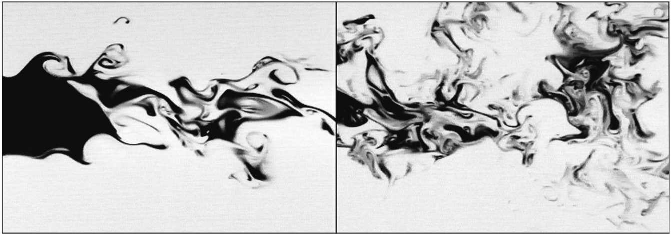
FIG. 1. Instantaneous planar cuts of the scalar field (disodium fluorescein in water, Sc=2000 ) downstream of the injection point illustrating how a scalar blob, initially compact and smooth, is progressively converted into disjointed sheets with broad fluctuations in thickness and concentration. d=1 cm. Left: the picture covers the region just downstream of the injection tube 0 < x/d < 4 . Right: further downstream 4 < x/d < 8 .
