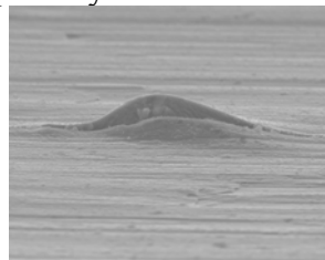
Fig. 10: Plan view of a short crack initiated at a surface bulge. The bulge was formed by the oxidation of a sub-surface (Nb,Ti)C primary carbide.
