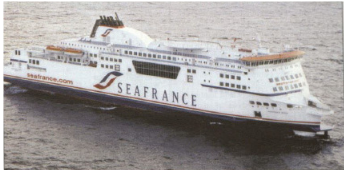
The 33,796gt SeaFrance Rodin , with a service speed of 25knots, brings a new dimension to passenger and ro-ro services between Dover and Calais. The 'cow-catcher' at the bow - a typical feature of Dover/Calais ferries - is designed to speed mooring at the shore ramps.
