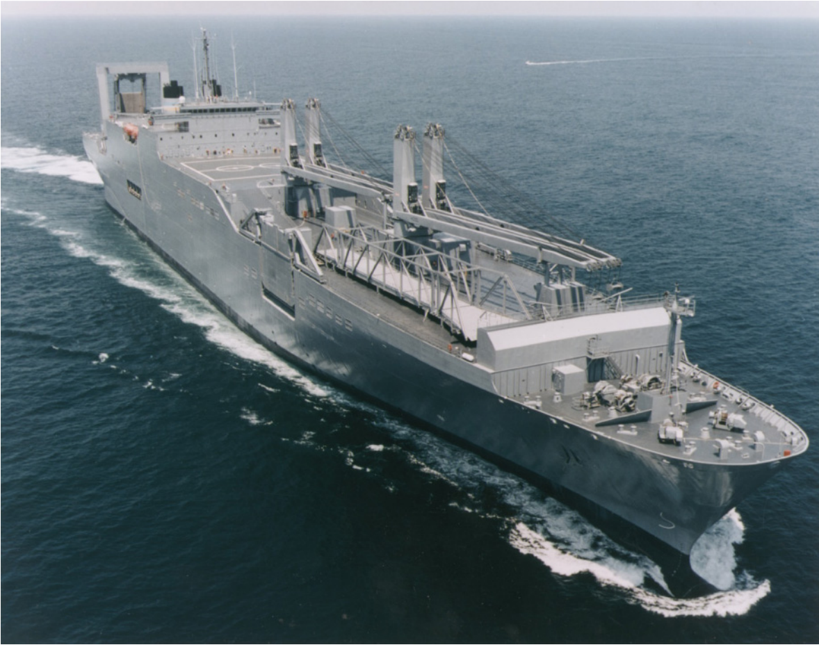
Figure 7.2: USNS GORDON (T-AKR 296) Note sideport/aft ramps & cargo cranes www.msc.navy.mil
