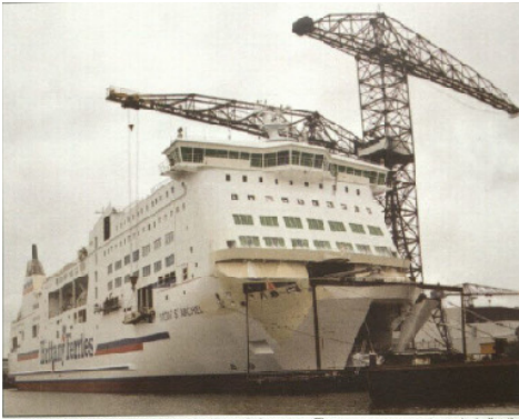
Mont St Michel nearing completion at the outfitting quay. The ro-ro access package, including the clam doors seen here, was supplied by the MacGregor group. Three fixed vehicle elevators are available, together with hoistable platforms on the upper deck.
