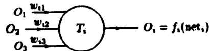
Figure 14. A sketch of the i th formal neuron. This neuron has 3 inputs: the output from neuron 1, O_1 , from neuron 2, O_2 , and from neuron 3, O_3 . Each of these inputs is weighted with an individual weight, w_{11} , w_{12} , w_{13} , respectively. The output from this neuron, O_i , is here given by f_i(net_i = \sum_{j=1}^3 w_{ij} O_j - T_i) .
