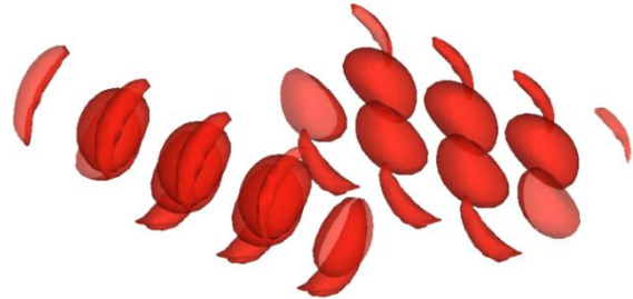
Figure 9: a 3D extrapolation of the perturbation vorticity field at relatively distant vortex spacing a/b=0.251 . Vorticity of each iso-surface is \omega_z=4.0 Note the sinusoidal nature of the perturbation fields with the pairs of vortices seen in figure 8a).
