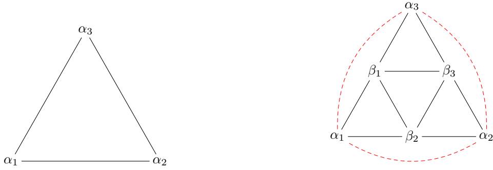
(a) A face of the icosahedron not subdivided, k = 0 . (b) A face of the icosahedron subdivided once, k = 1 .
