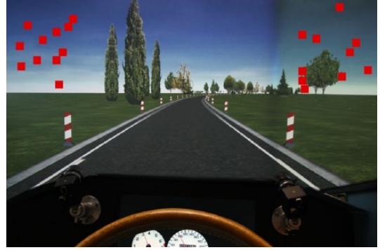
Figure 2. Photo of the driving simulator. The superimposed squares indicate the positions where visual stimuli could appear.
