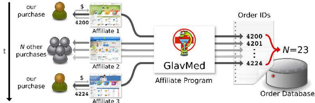
Figure 1: How the purchase pair technique works. In this hypothetical situation, two measurement purchases are made that bracket some number of intervening purchases made by real customers. Because order number allocation is implemented by a serialized sequential increment, the difference in the order numbers between measurement purchases, N = 23 , corresponds to the total number of orders processed by the affiliate program in the intervening time.
