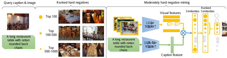
Fig. 3. Moderately hard negative mining. The left part shows a ground-truth caption and its top hard negatives mined from unlabeled images. The right part shows the process of moderately hard negative mining. The circles of different sizes stand for the similarities between each image and the query caption.
