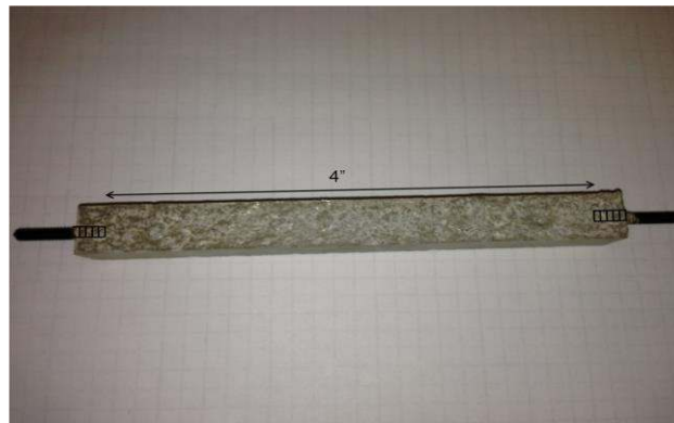
Figure 4-1. “Mini-bar” cast for drying shrinkage
