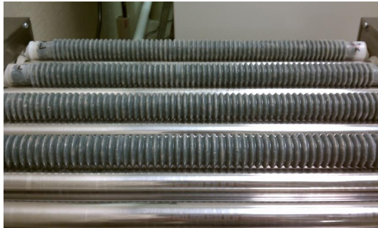
Figure 3-3. Corrugated polyethylene cylindrical molds for autogenous shrinkage measurement
