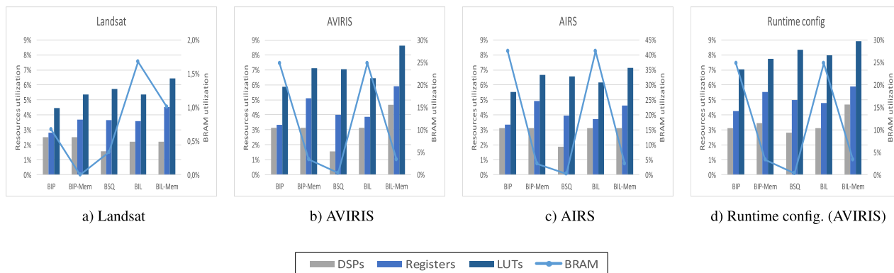
FIGURE 10. CCSDS123 IP- Synthesis results on Xilinx Virtex5QR XQR5VFX130.
