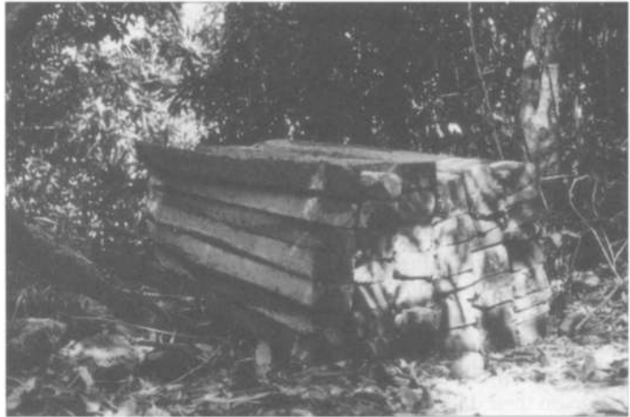
Cut and squared timbers ready for shipment to Atlas Mining Company, Masbate Island. Each timber measures 6" × 8" × 8' (15 cm × 20 cm × 2.4 m) (N. R. Ingle).
