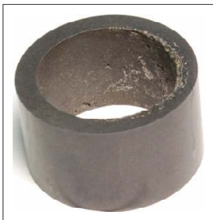
Fig. 13 – SiC p /Al 2 O 3 ceramic matrix composite hollow cylinder fabricated in the present work (inside diameter = 30 mm, outer diameter = 40 mm, thickness = 5 mm)
