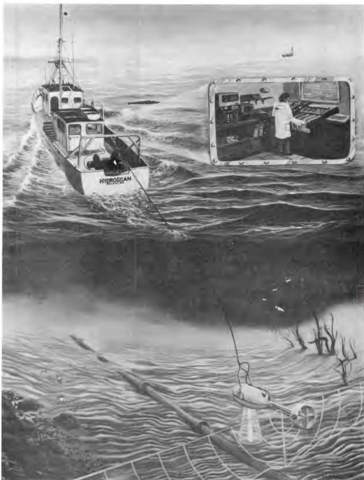
Figure 2. Components of a typical side-scan sonar system (Courtesy of Klein Associates, Inc.)
