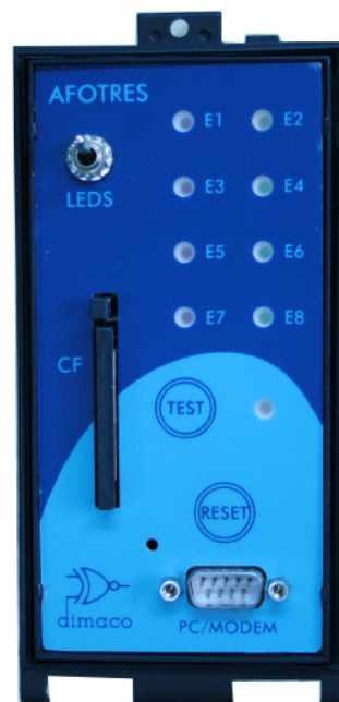
Figure 2. Eight-loop vehicle inductive detector (Afortres–Dimaco).
