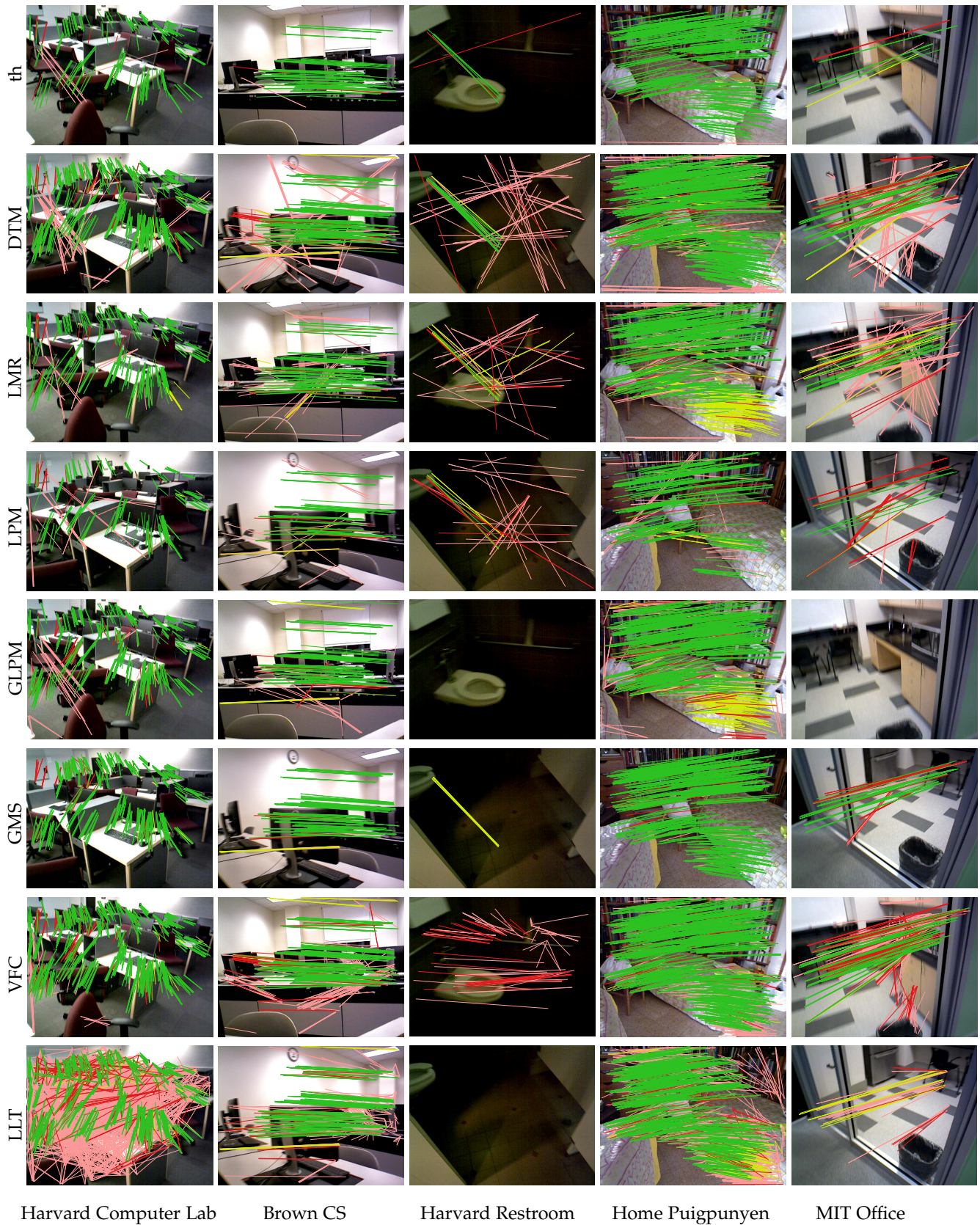
Fig. 19. SUN3D local spatial filter matches according to the best configuration setup, the images of the input pair alternate among the rows. For each method inlier (yellow, green) and outlier (red and light red) clusters are shown, as well as the 1SAC filtered matches (green, red) (see Sec. 5.3, best viewed in color and zoomed in).
