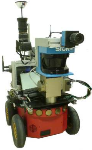
Fig. 4. The mobile robot platform, used to acquire the images used in this paper. The omnidirectional camera can be seen in the top left part of the image.
