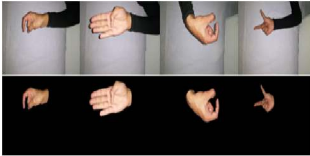
FIGURE 2: Segmentation of PSL signs with different scaling, illumination and rotation
