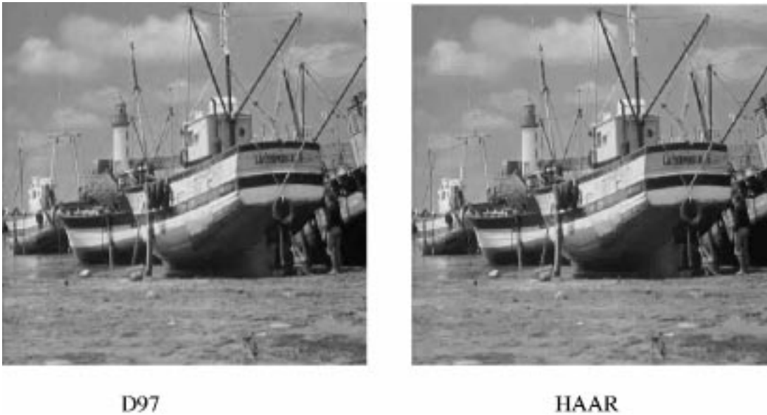
Fig. 4. Image “boat” has been compressed to 0.5 bits/pixel. (a) Image “D97” uses the Daubechies (9, 7) wavelet and (b) image “HAAR” uses the HAAR wavelet.
