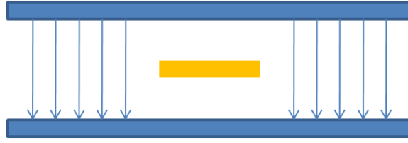
Figure 88. Parallel plate mode of propagation in stripline with non-ideal references.
