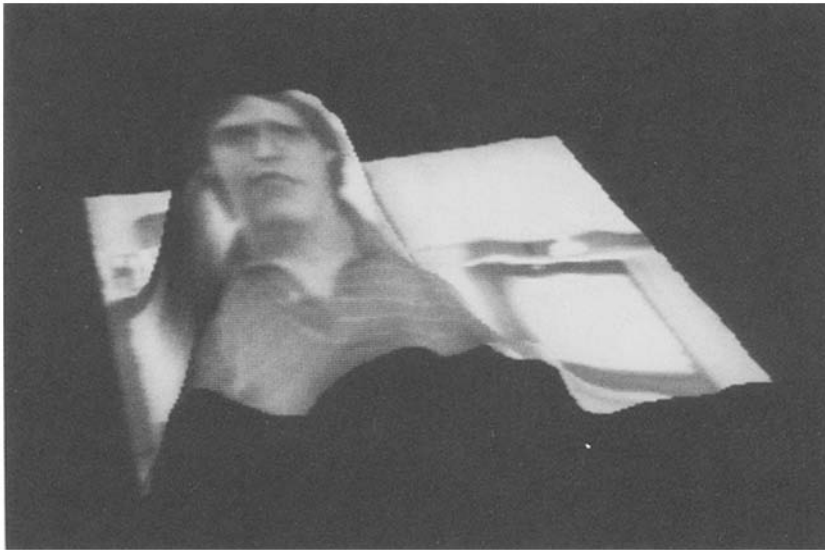
Fig. 3. Two frames from a motion sequence (a). The original image has been texture mapped onto a surface that encodes speed as elevation (b). The raised area indicates motion before a stationary background.
